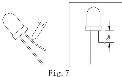
2) Forming lead should be carried out prior to soldering and never during or after soldering.
